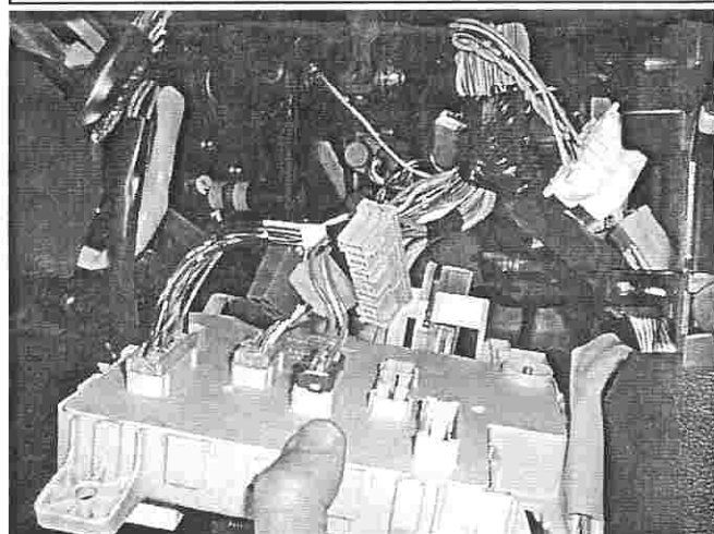
Fig 3. Grey 18 pin connector unplugged from the fuse panel.
