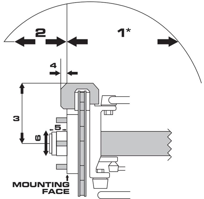
\* Measure backspace to first point of contact look carefully up and down for the first point at the rear this is often leaf spring.
