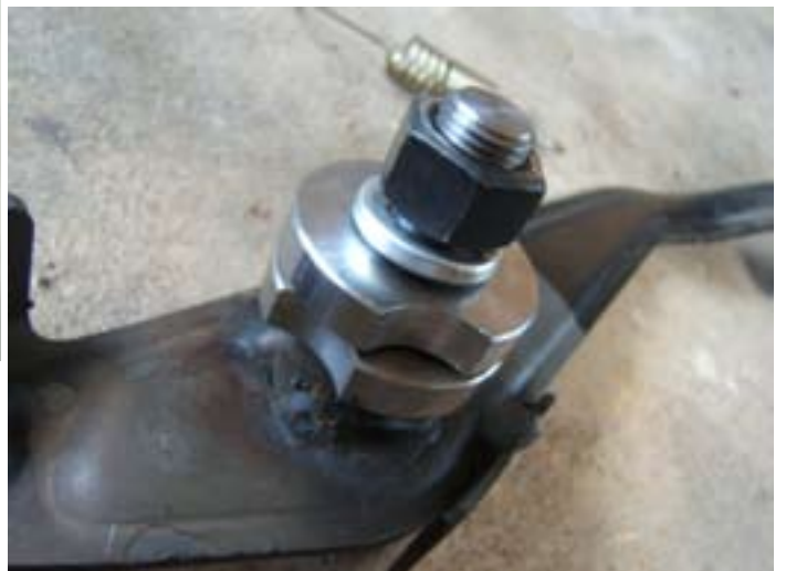
This is the clip that the clutch cable joins on to
