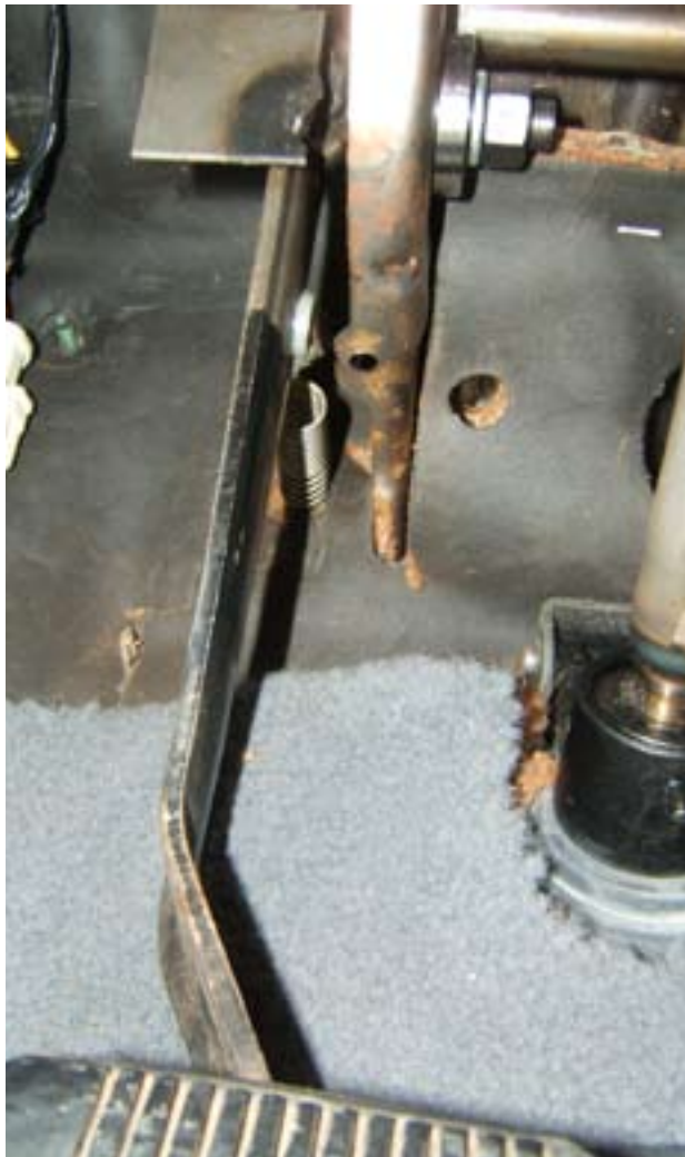
Install Mal Wood clutch pedal pin onto clutch pedal as shown.
