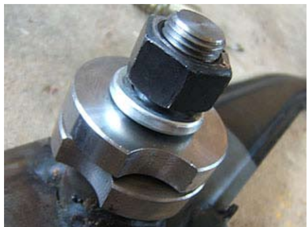
Install Mal Wood clutch pedal pin onto clutch pedal as shown.
