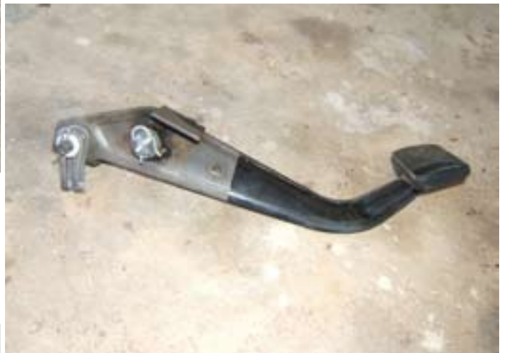
This is the clip that the clutch cable joins on to
