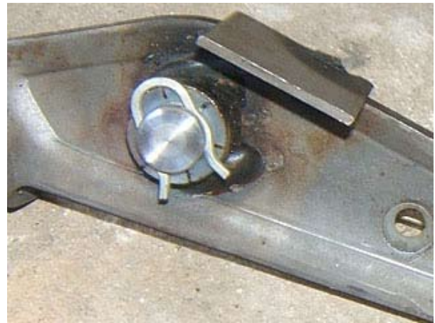
Install Mal Wood clutch pedal pin onto clutch pedal as shown.
