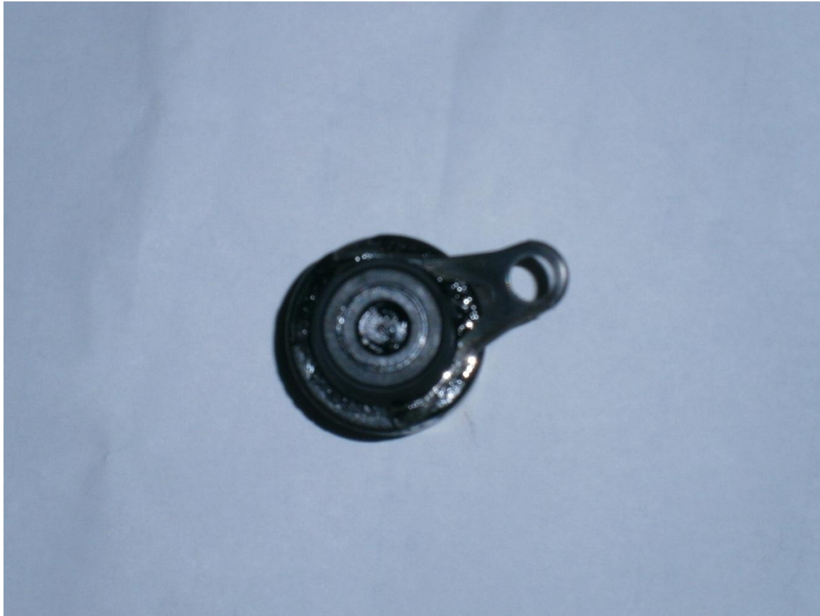
End on view of solenoid- depicting oblong within throat.
