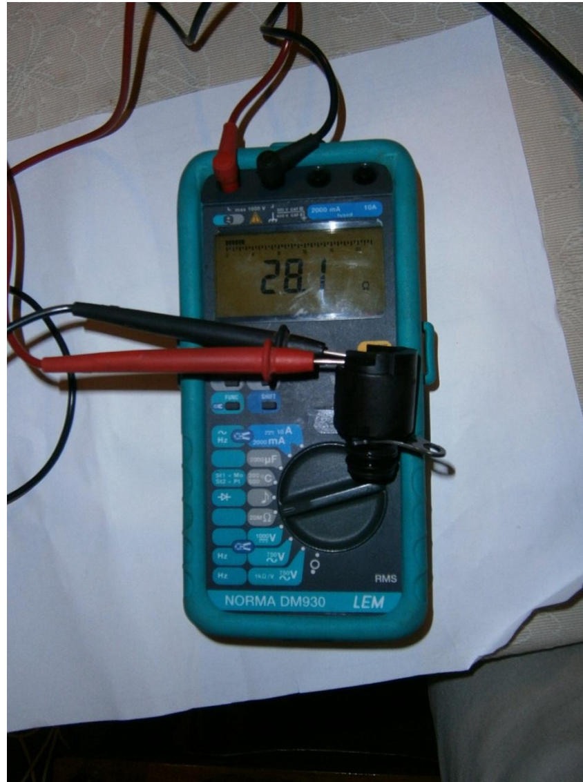
Measurement of shift solenoid coil resistance 28.1Ω
