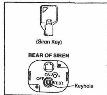
The alarm system can be disabled using the siren key supplied.
